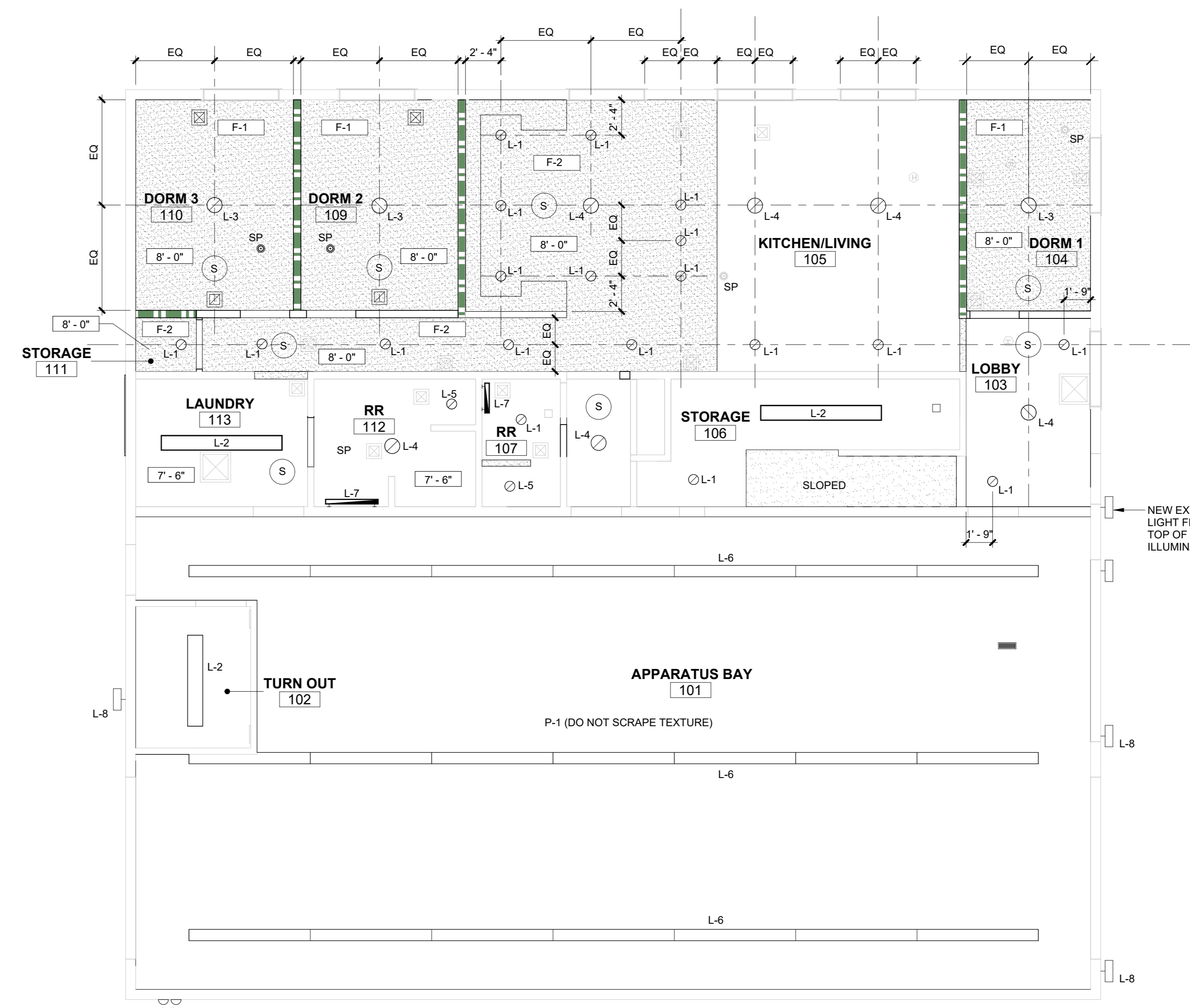
3 FIRST FLOOR REFLECTED CEILING PLAN 3/16" = 1'-0"
