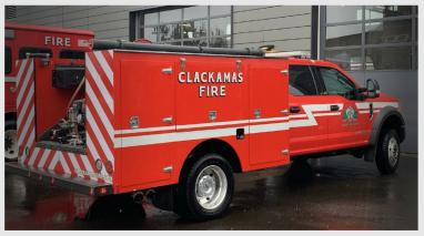
think about is how these essential tools that support the mission can arrive quickly. That is the advantage of a Quick Response Unit (QRU). These QRUs may also be set up to handle several types of critical incidents. A QRU is a smaller vehicle that allows us a quicker initial response to calls for service and improves efficiency in highvolume service areas.
