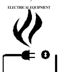
Type C extinguishers fight energized electrical fires such as burning wires, fuse boxes, circuit breakers, machinery, and appliances.
